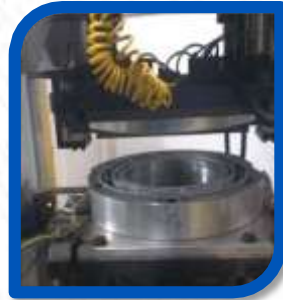
Hot Plate Welding
